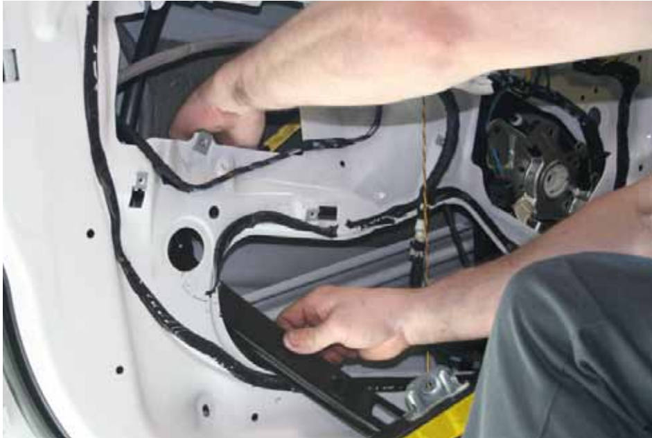
Quite a bit of disassembly is necessary to work on a malfunctioning window regulator.
