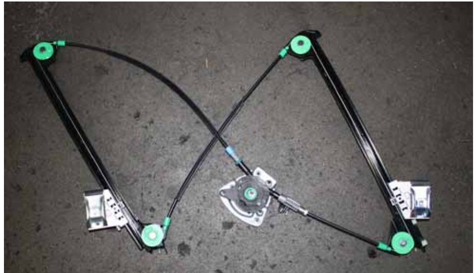
Cables and pulleys make up the newest window regulator configuration for our modern Porsches. In this example (from a 996), the window glass fits into the two metal clips and the motor attaches to the hub in the center of the picture. The cables do the lifting.
