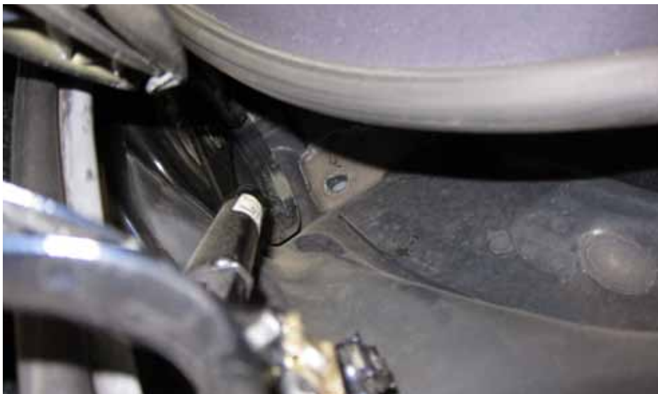
Shown here: the convertible top drain hole on a 987 Boxster. By partially lowering the top so that the tonneau is raised, you can access these drains at the lowest point in the top storage bucket. The drain is the circular opening in the center of the photo. There is one on each side of the car.
